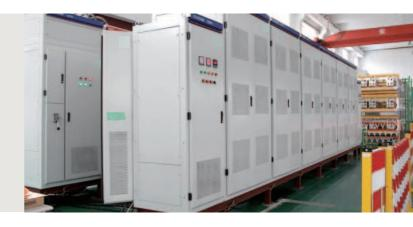
The Static Synchronous Compensator is a voltage regulating device based on voltage source converters (MOSFET). It acts as a source or a sink of reactive power which is independent of ac system voltage. STATCOM can operate as a part of Flexible AC Transmission System (FACTS) to detect and compensate voltage fluctuations or flickers instantly, correct unbalanced loads and control power factor.
